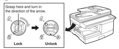
To lock the scan head locking switch, hold up the catch in illustration (A) and turn the center knob counter-clockwise 90 degrees until you hear a click.
